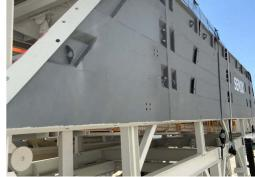
With trapezoidal bending for aggregate bin covers a high strength can be reached. In SEMIX's aggregate storage hoppers, extra reinforcement steels are welded to the empty spaces in the trapezoid. Thanks to this method, aggregate storage bins can serve long years.
