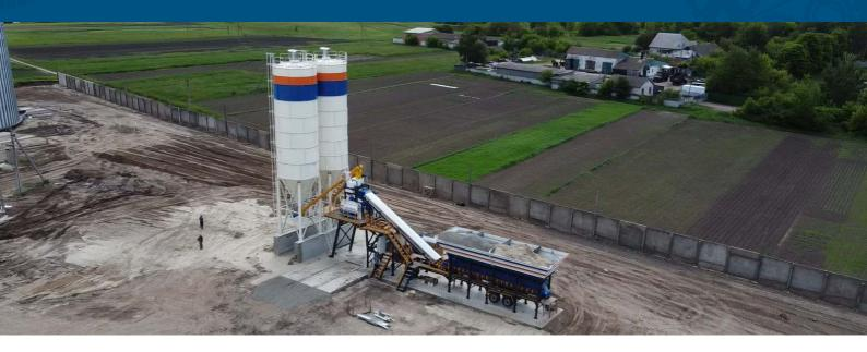
SEMIX Mobile 90S5 is equipped with 2250/1500 liters capacity Concrete mixers which can be a single shaft, twin shaft, or planetary type mixers. In SEMIX Concrete Mixers NiHard4 or Hardox 450 wearings are used according to the Concrete recipe's sillicium ratio.
