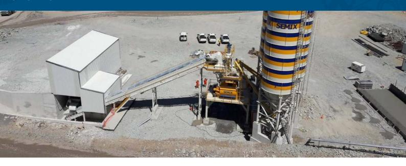
SEMIX Stationary 160 is equipped with 6750/4000 liters capacity Twin Shaft Concrete mixers. In SEMIX Concrete Mixers NiHard4 or Hardox 450 wearings are used according to the Concrete recipe's sillicium ratio.
