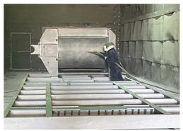
All components of the SEMIX's concrete batching plants are treated with Grit Blasting process in SEMIX's certified grit blasting facility before the painting with steel balls. This method provides high surface finish quality after the painting.
