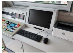
Air conditioner, electrical connections and lightening - present at control cabin. Power board with manual control system provides production options completely at automatic mode as well as manual mode. Power board includes safety system protection switches for motors (phase protection relay), circuite breaker in case of overload. All electrical components are SCHNEIDER brand. Full set of computer for automation system with printer/UPS - present.
