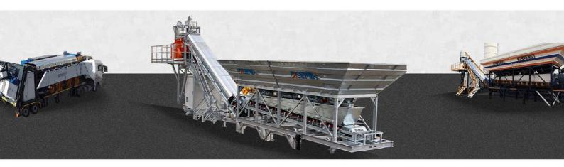
SEMIX Mobile 60 S4 is equipped with 1875/1250 liters capacity Concrete mixers which can be a single shaft or 1500/1000 planetary type mixers. In SEMIX Concrete Mixers NiHard4 or Hardox 450 wearings are used according to the Concrete recipe's sillicium ratio.
