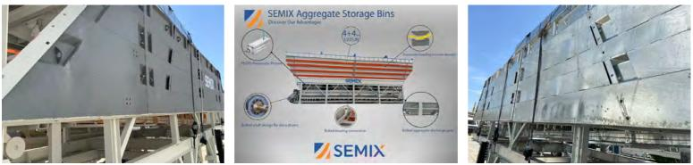
With trapezoidal bending for aggregate bin covers a high strength can be reached. In SEMIX's aggregate storage hoppers, extra reinforcement steels are welded to the empty spaces in the trapezoid. Thanks to this method, aggregate storage bins can serve long years.
