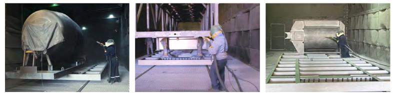
All components of the SEMIX's concrete batching plants are treated with Grit Blasting process in SEMIX's certified grit blasting facility before the painting with steel balls. This method provides high surface finish quality after the painting.
