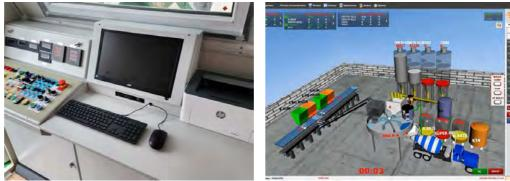
Air conditioner, electrical connections and lightening - present at control cabin. Power board with manual control system provides production options completely at automatic mode as well as manual mode. Power board includes safety system protection switches for motors (phase protection relay), circuite breaker in case of overload. All electrical components are SCHNEIDER brand. Full set of computer for automation system with printer/UPS - present.
