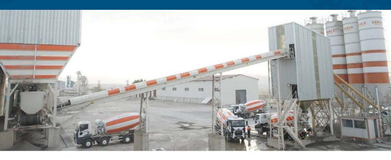
SEMIX Stationary 240 is equipped with 9000/6000 liters capacity Twin Shaft Concrete mixers. In SEMIX Concrete Mixers NiHard4 or Hardox 450 wearings are used according to the Concrete recipe's sillicium ratio.
