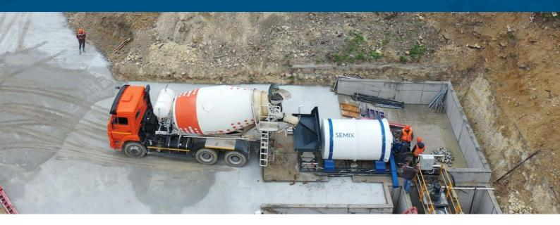
Recycling system SEMIX SMRC 15 Rotating Body of Recycling System Motor Power of Body : 2.2 KW x 2 pcs.
