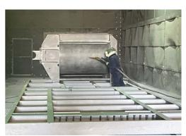
All components of the SEMIX's concrete batching plants are treated with Grit Blasting process in SEMIX's certified grit blasting facility before the painting with steel balls. This method provides high surface finish quality after the painting.
