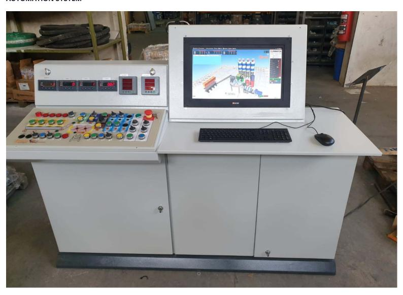
**Production Screen;**You can monitor process of the operation on the animation screen, which is infrastructure by Microsoft DirectX. During the producing, required values, measurement values and differences of values will be shown. Following of the measured will be checked by the system during the process and it will be shown on automation screen with error sound if there is a problem. It can add or discharge water automatically without changing value of cement, during the process.
