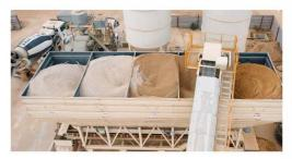
Aggregate Bins Capacity & Quantity: 3 x 11 m3 (Linear)
