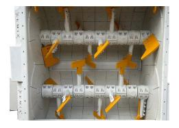
Mixing Blade: Ni-Hard 4 (Chrome, Nickel special alloy cast iron)
