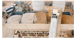
Aggregate Bins Capacity & Quantity: 3 x 17 Tons (Linear) LOW PROFILE DESIGN
