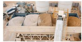
Aggregate Bins Capacity & Quantity: 3 x 20 m³ (Linear)
