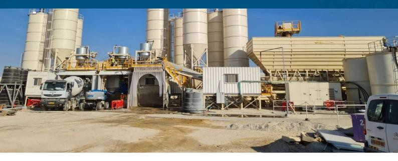
SEMIX Portable Dry Concrete Batching Plants S120D is equipped with cement, aggregate, water and admixture batchers for an output of 150 yd<sup>3</sup>/h.
