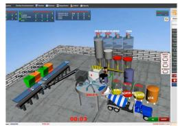
**Production Screen;**You can monitor process of the operation on the animation screen, which is infrastructure by Microsoft DirectX. During the producing, required values, measurement values and differences of values will be shown. Following of the measured will be checked by the system during the process and it will be shown on automation screen with error sound if there is a problem.
