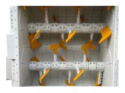
Mixing Blade: Ni-Hard 4 (Chrome, Nickel special alloy cast iron)
