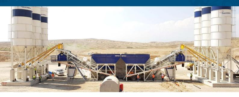
SEMIX Mobile 60V is equipped with 1875/1250 liters capacity Concrete mixers which can be a single shaft, twin shaft, or planetary type mixers. In SEMIX Concrete Mixers NiHard4 or Hardox 450 wearings are used according to the Concrete recipe's sillicium ratio.
